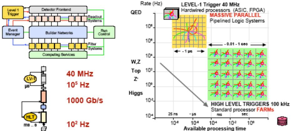
L1 gets us from 40MHz to 100kHz using a fixed  $3\mu s$  to decide. HLT gets us from 100kHz to 100Hz using 0.01-1sec to decide.
